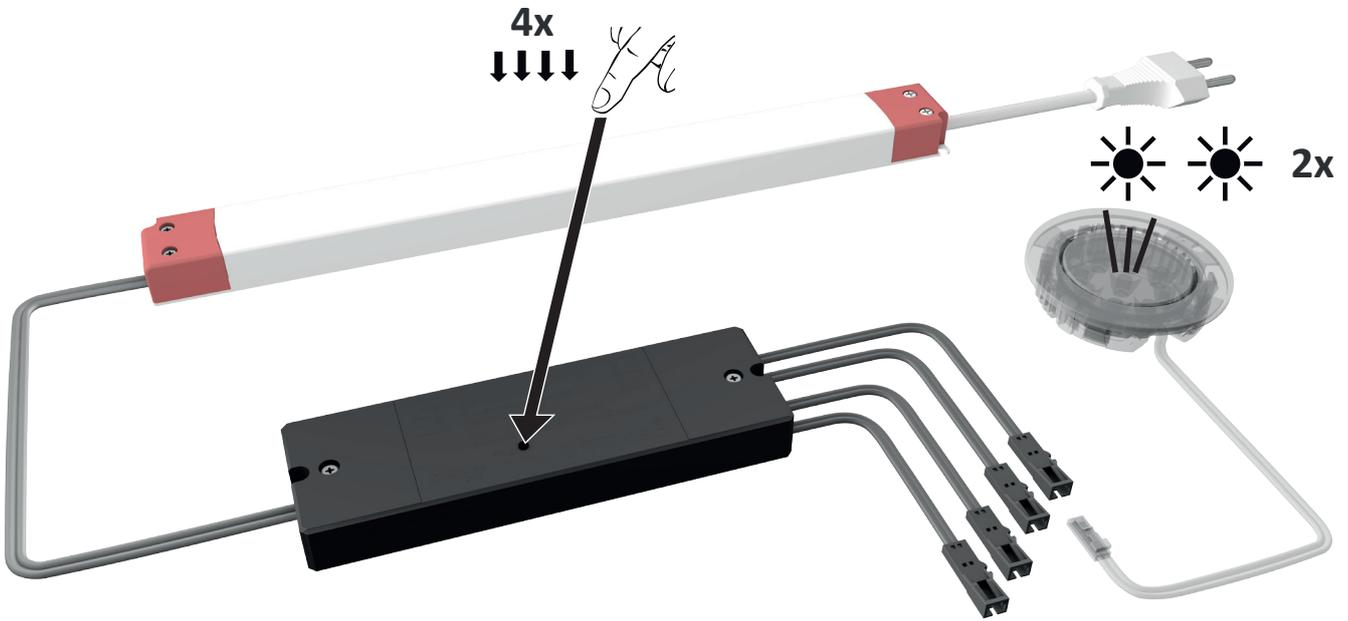
**Factory reset – Remove all connections to start a new configuration
